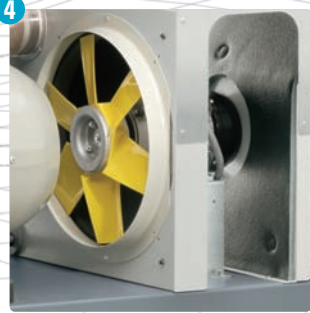
Controlled cooling fan
